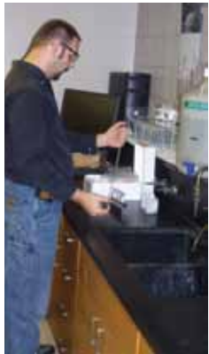
Lab staff at the Grandville, MI, Wastewater Treatment Plant now use prepackaged vial chemistries to streamline ammonia and phosphorus analysis for process control and permit reporting.
